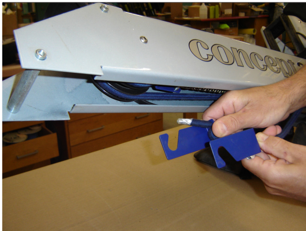
1. Remove the footplate covers by taking out the 12 philips head screws.
