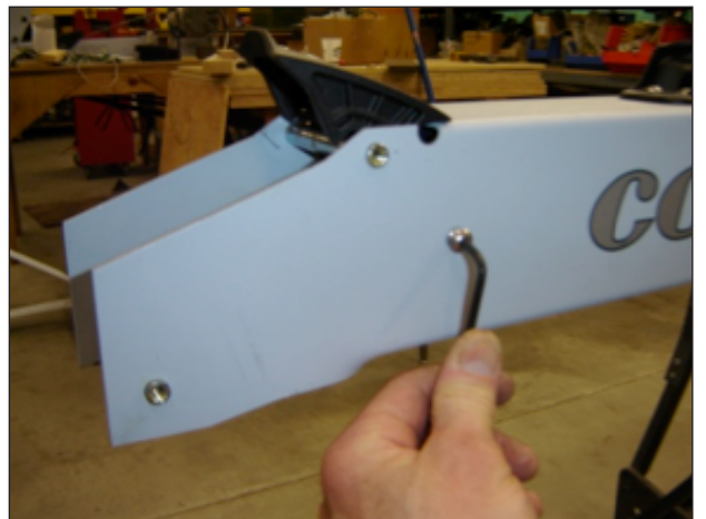
2 & 3. Remove the footplate bellies by taking out the 4 7/16" hex screws and plates.
