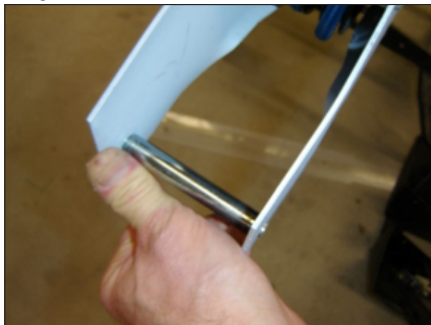
4. Detach the two shock cord SCAMS to relieve bungee tension.
