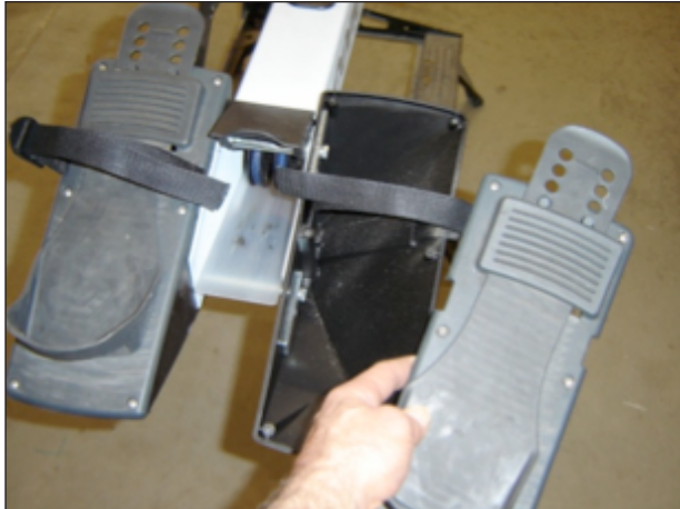
1. Remove the footplate covers by taking out the 12 philips head screws.
